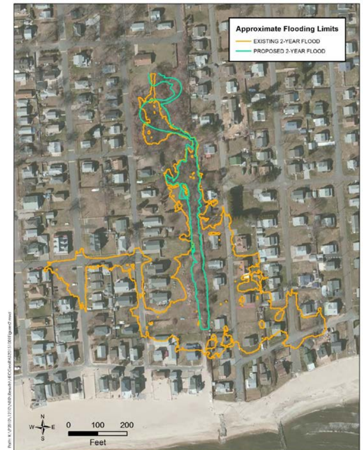
Figure 3-8 HEC-RAS Modeled Proposed Conditions (with Twin Culverts) 2-Year Flood Extents
